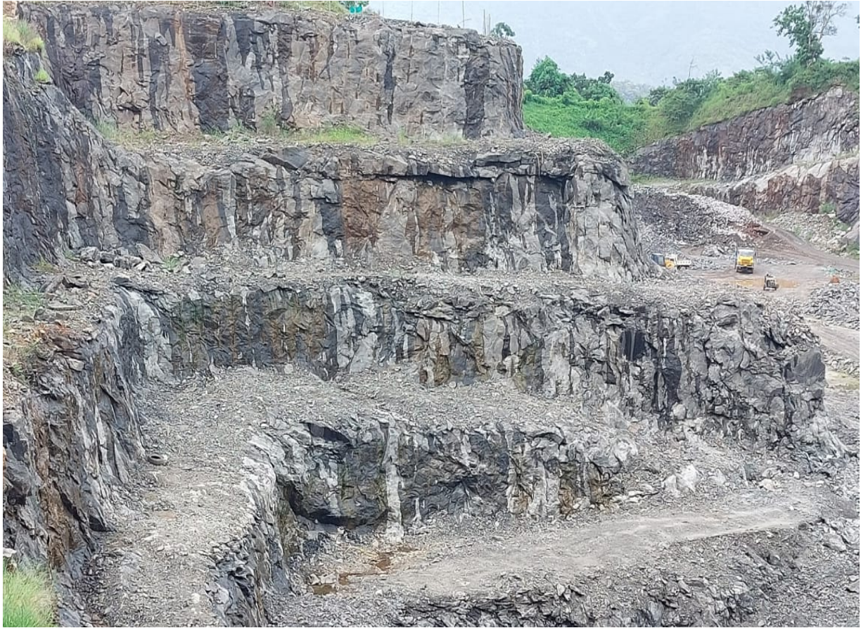
PHOTOGRAPHS SHOWING FORMATION OF BENCHES
