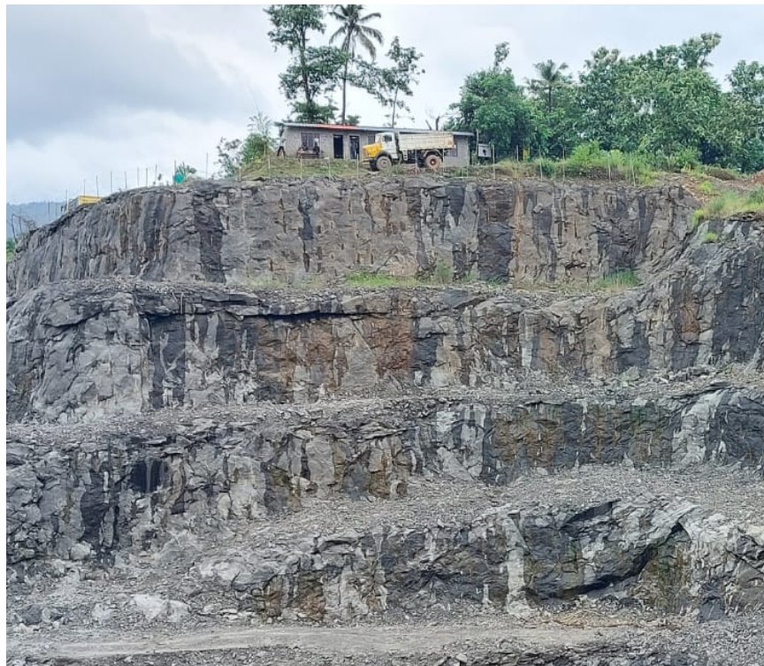
PHOTOGRAPHS SHOWING FORMATION OF BENCHES
