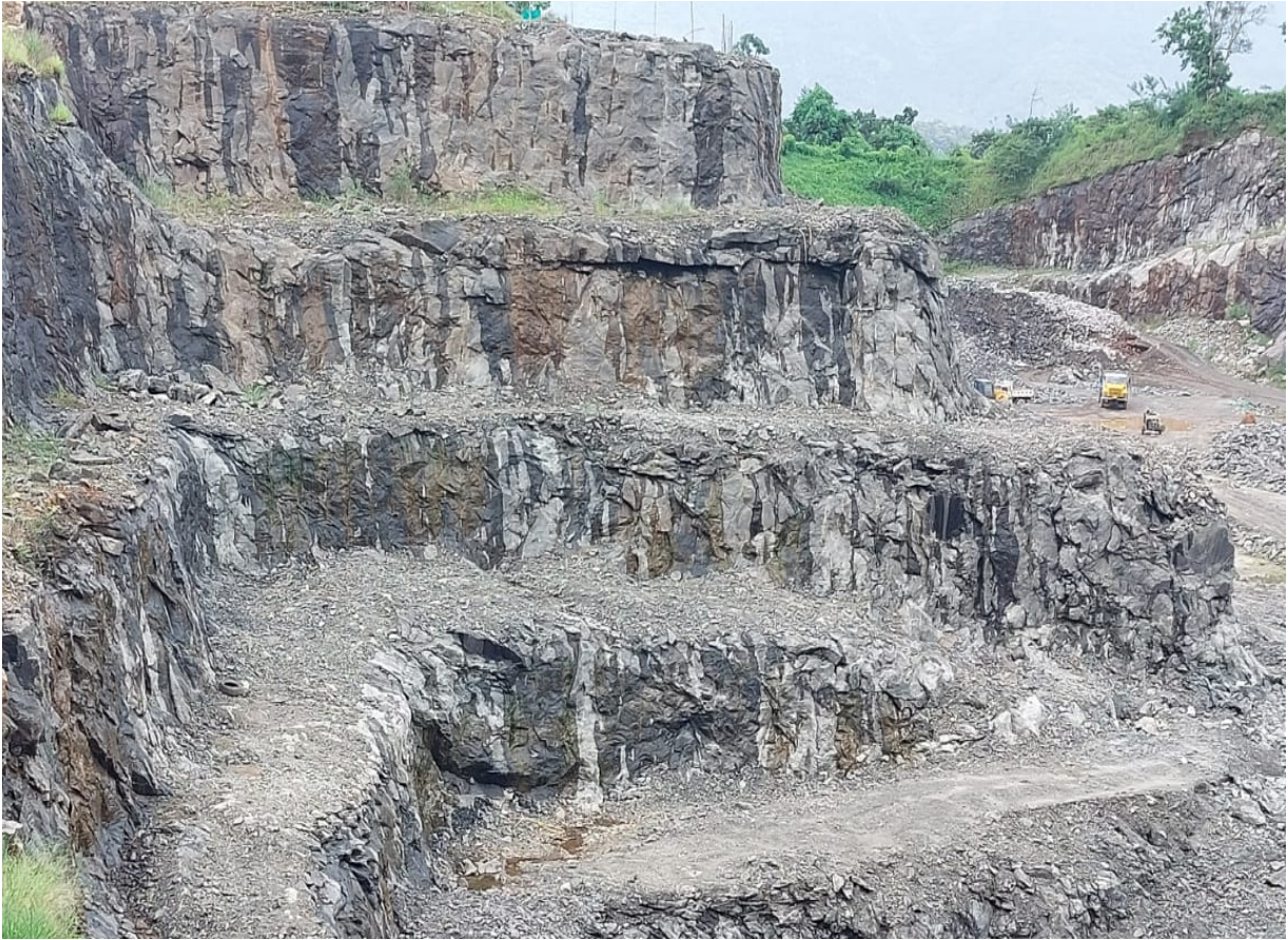
PHOTOGRAPHS SHOWING FORMATION OF BENCHES
