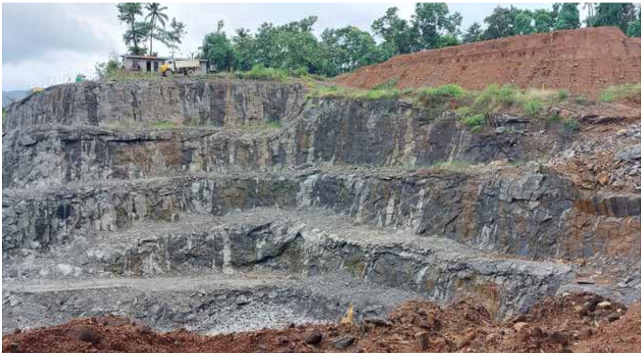
PHOTOGRAPHS SHOWING FORMATION OF BENCHES
