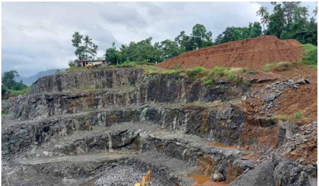
PHOTOGRAPHS SHOWING FORMATION OF BENCHES
